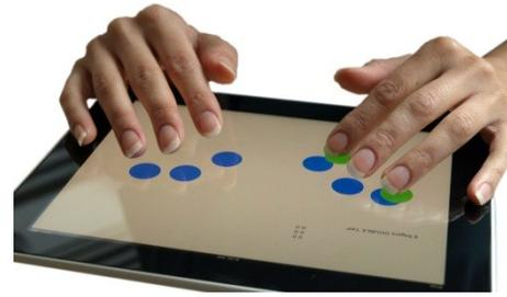
**Figure 5. Perkins-style keyboard on a tablet.**
