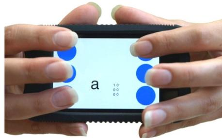
Figure 1. BrailleTouch on a smartphone.
